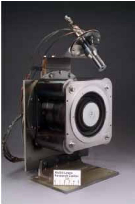
Figure 3 - D-80 High Specific Impulse Two-Stage Hall Thruster
