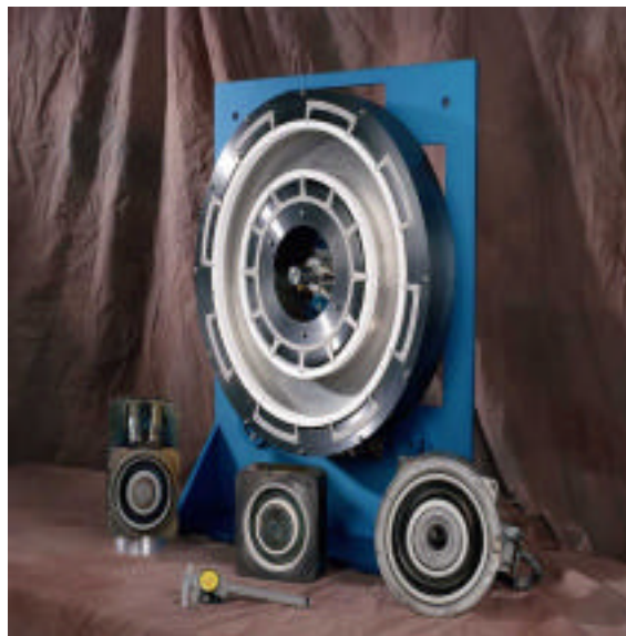
Figure 1 – NASA-457M (large thruster in the center), NASA-120M (small thruster in the center), SPT-100 (left), T-160E (right).
