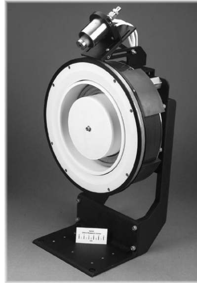
Figure 1 - Photograph of the NASA-173Mv2 Hall thruster.
