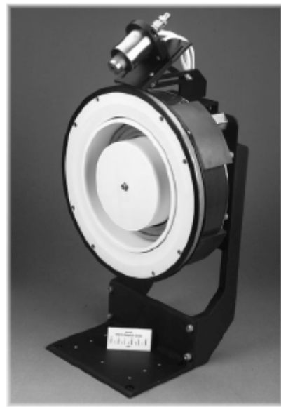
Figure 1 - Photograph of the NASA-173Mv2 Hall thruster.
