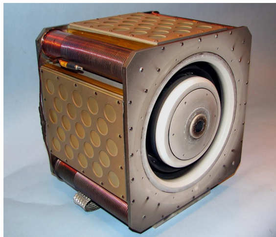
Figure 2. Photograph of the laboratory-model 8 kW Busek BHT-8000 Hall thruster.
