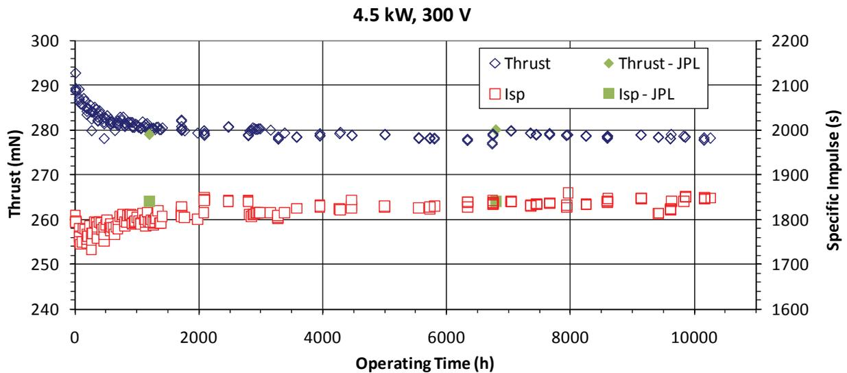
**Figure 5. Comparison of the measured thrust and specific impulse from the life test QM thruster and values measured at JPL on an EM thruster with insulator rings pre-machined to the erosion geometry after 1,200 or 6,800 h (steady-state) of operation.**
