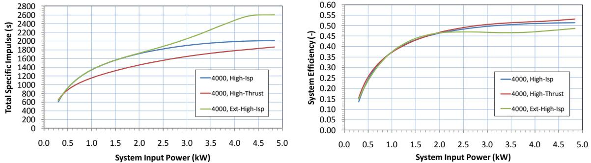
Figure 11. Specific impulse and efficiency for various BPT-4000 throttle curves.
