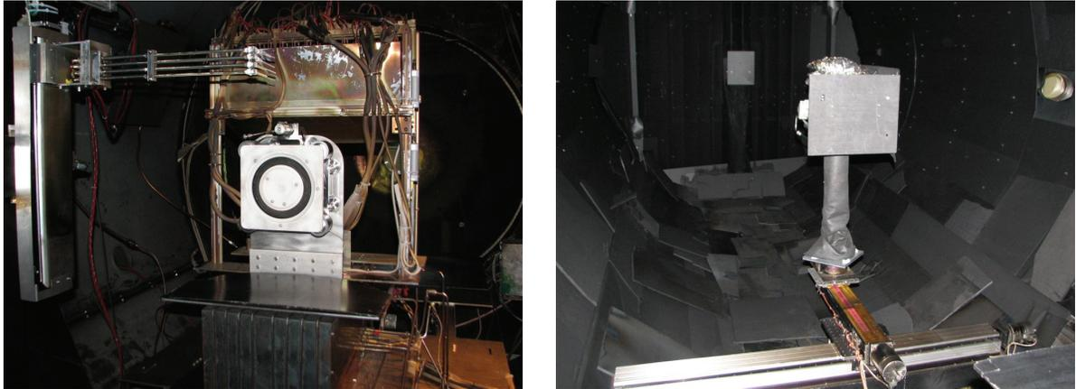
Figure 1. Photographs of the experimental configuration showing the thruster installed on the thrust stand (left) and the far-field plume probe array (right).
