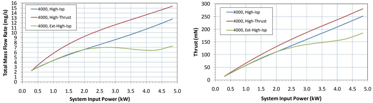
Figure 10. Mass flow rate and thrust for various BPT-4000 throttle curves.
