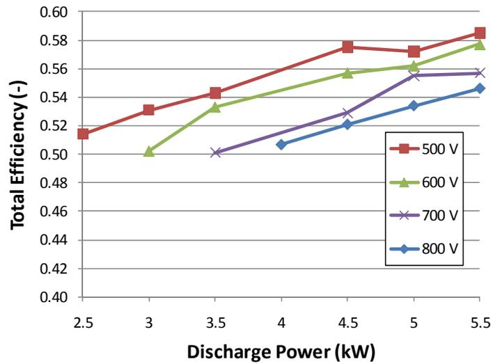
Figure 6. Thrust, specific impulse, and efficiency of the BPT-4000 operating over 500-800 V, 2.5-5.5 kW.
