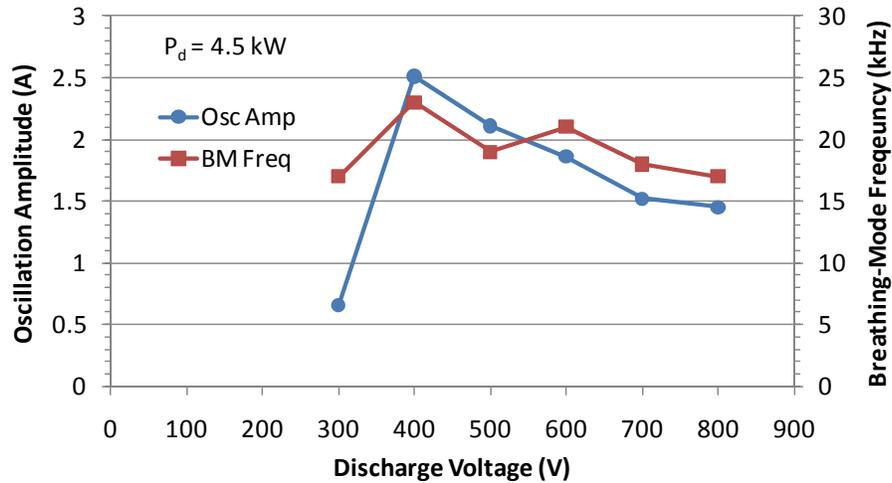
Figure 7. Oscillation amplitude and breathing-mode frequency from the discharge current probe on the anode side of the discharge.
