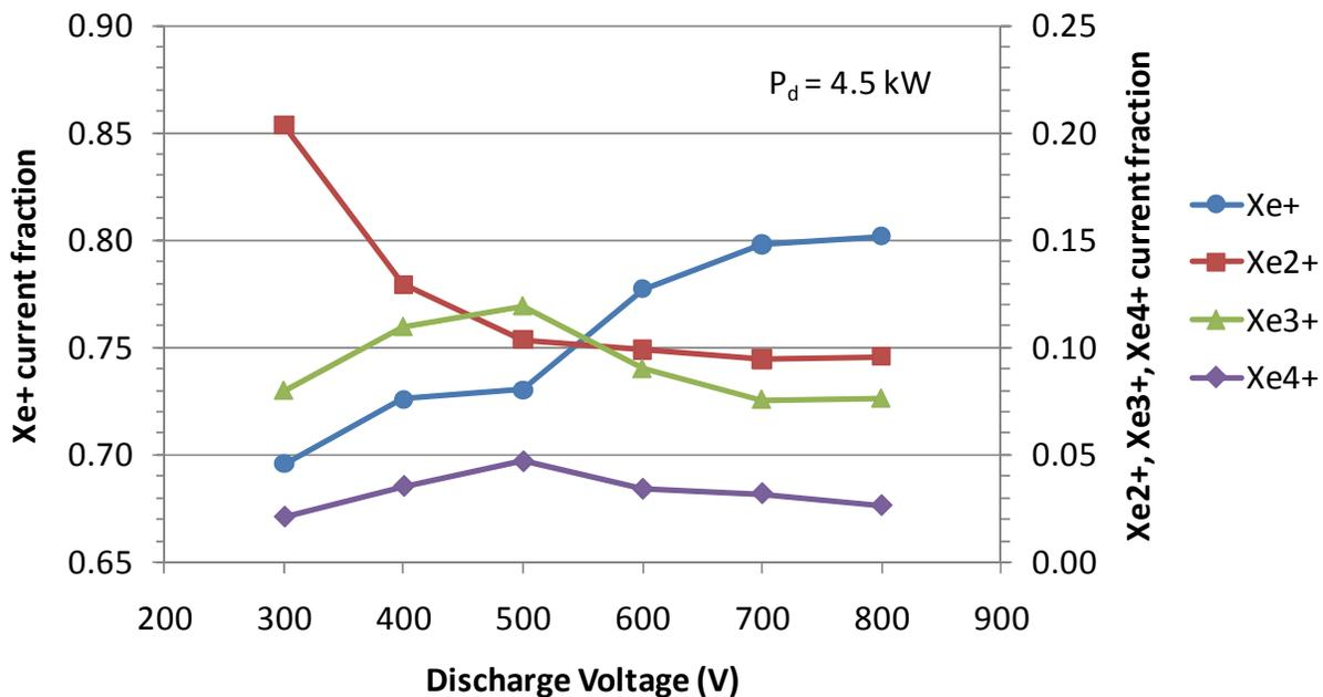
Figure 9. Ion species' current fractions measured with the ExB probe for operation over 300-800 V, 4.5 kW.
