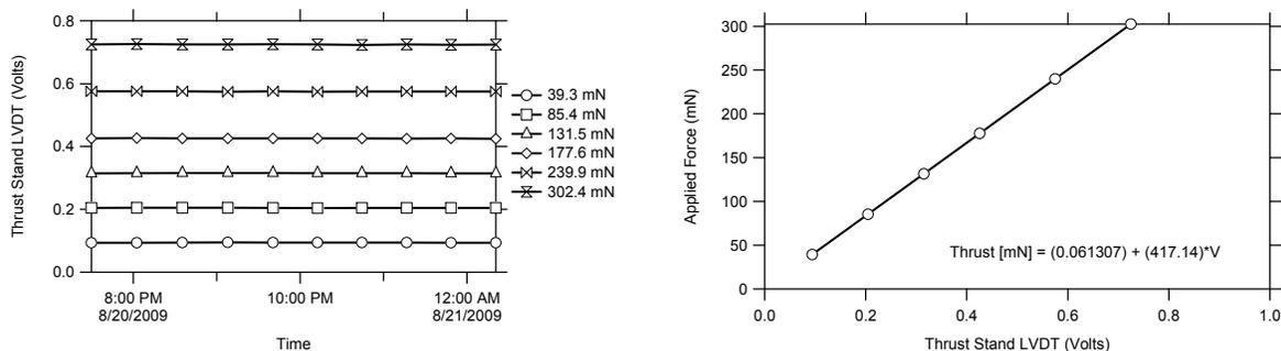
**Figure 3. Thrust stand calibration results. Left: LVDT response to calibration weights. Right: Thrust stand calibration curve.**
