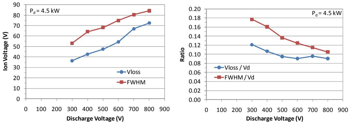
Figure 8. Ion loss voltage and full-width at high-maximum (FWHM) as measured with the RPA for operation over 300-800 V, 4.5 kW. Left: Loss voltage and FWHM in absolute terms. Right: Loss voltage and FWHM as a fraction of the discharge voltage.
