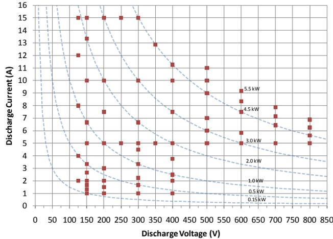
**Figure 4. Operating conditions investigated over the course of all experiments conducted at JPL. Lines of constant discharge power are drawn for reference. Current, voltage, and power throttling ranged from 1-15 A, 125-800 V, and 0.15-5.5 kW, respectively. In this paper, the focus is on operation from 500-800 V, 2.5-5.5 kW.**
