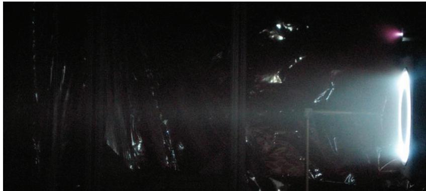
Figure 2. Operation of the BPT-4000 at 800 V, 4.5 kW.
