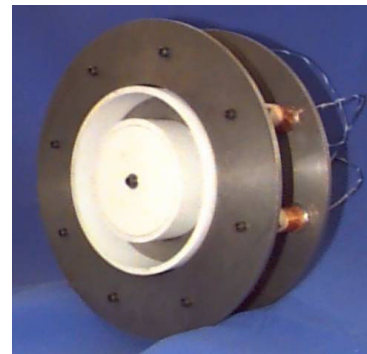
Figure 16 – Photograph of the single-stage P5, a nominally 5 kW laboratory model HET.
