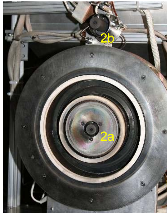
Figure 2. Laboratory Hall thruster with two \text{LaB}_6 hollow cathodes; 2a the internally mounted cathode and 2b the externally mounted cathode.
