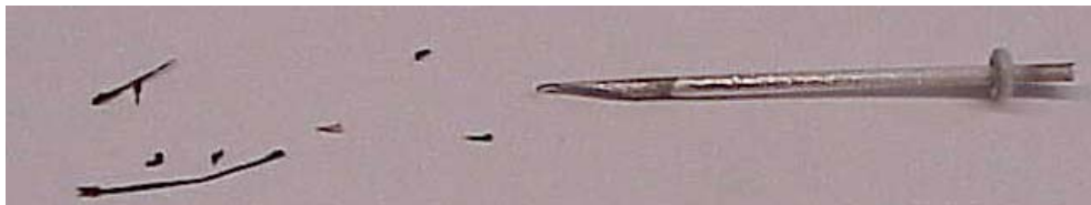
Figure 16. Mg wire after sublimation test, including shreds found in the vessel.
