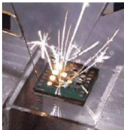
Fig. 19: Unintended multiple cavity firing in a digital micro-thruster array due to heat conduction across the wafer [37]
