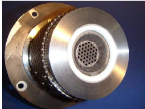
Fig. 26: The  $\mu$ NRIT-2.5 Miniature Ion Thruster of the University of Giessen [79]
