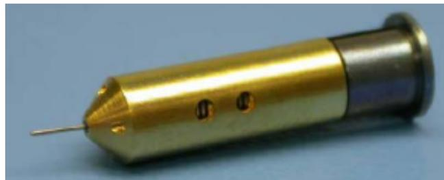
Fig. 31: Individual ST-7 Colloid Thruster Emitter [98]
