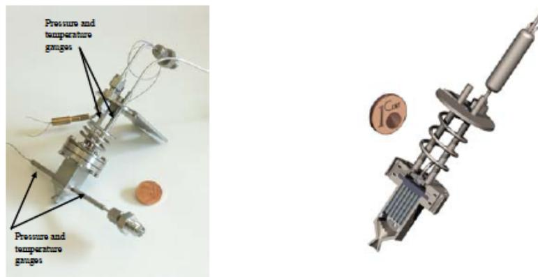
Figure 6: Miniature Hydrogen Peroxide Thruster by Scharlemann et al. [15]
