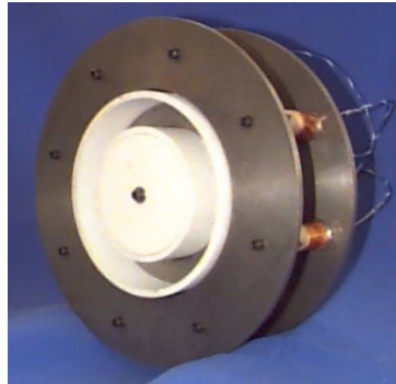
Figure 5-11 Photograph of the UM/AFRL P5 Hall thruster.
