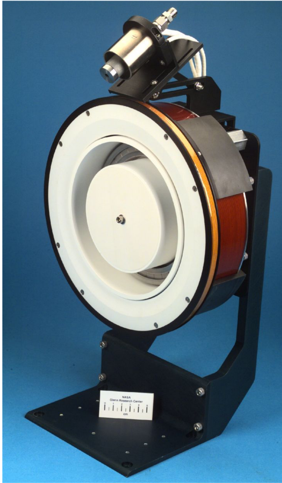
Figure 8-1 Photograph of the laboratory-model NASA-173Mv2 Hall thruster.
