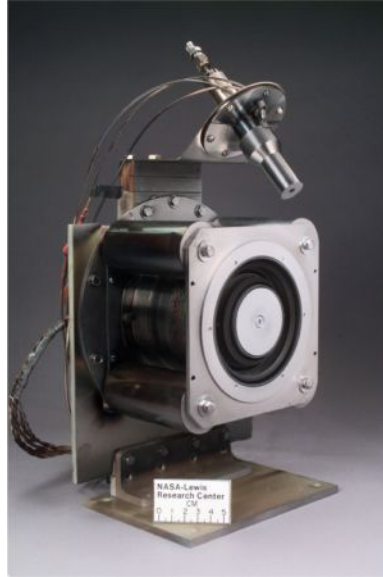
Figure 3-4 Photograph of a Hall thruster with a metallic discharge chamber, also known as an anode layer thruster. The thruster shown is the TsNIIMASH D-80, which is capable of single- and two-stage operation [132, 133].
